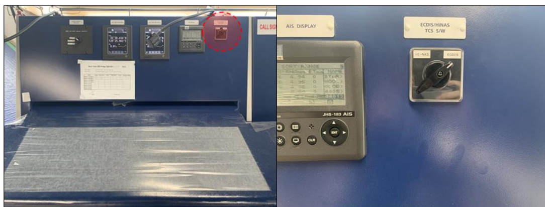
Figure 3: Hardware selector for switching between ECDIS TCS and HiNAS2.0
