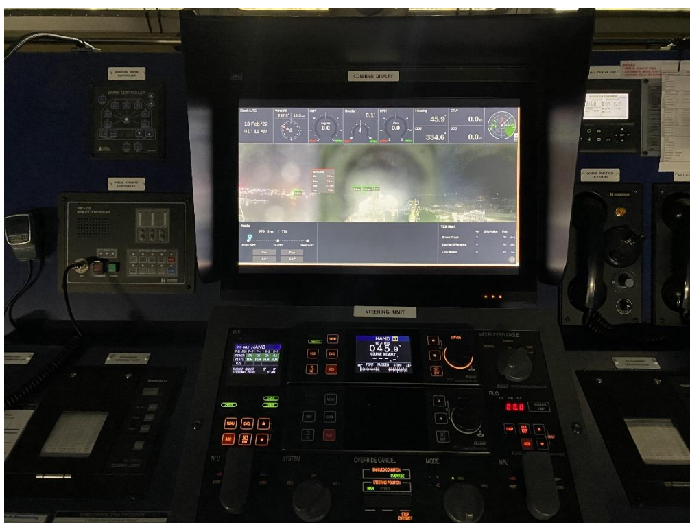
Figure 6: HiNAS2.0 display on Conning Display monitor at the centre console
